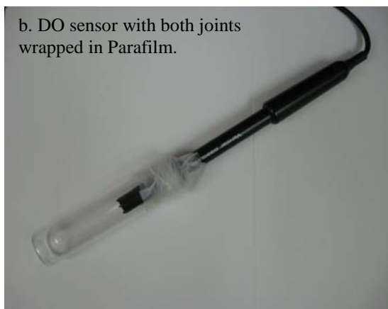
Figure 6. Graphic of Assembly of DO sensor and Vial for Overnight Data Recording.
