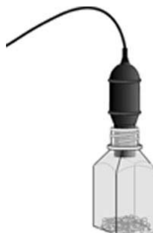
Figure 3. Set-up of O 2 sensor and Nalgene bottle for catalase reactions.
