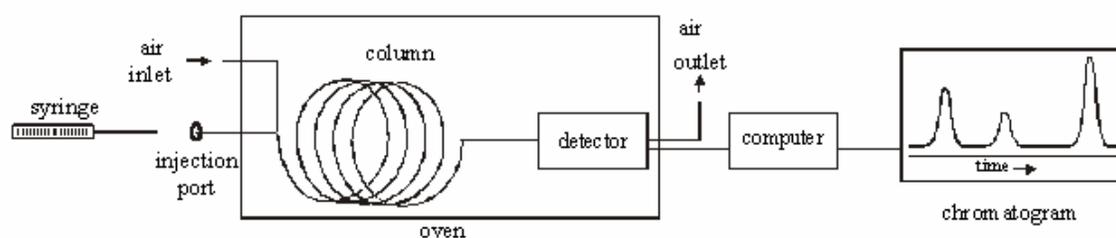
The gas chromatograph is an instrument that allows a chemist to separate a mixture of gases or volatile liquids. Separation is based on the size, structure, polarity of the molecules.
