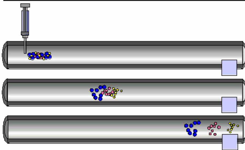
Retention time is used to identify the components, and the area under the curve is used to determine the relative quantities of the components. In this experiment, a HAYSEP-D column is used to separate ethanol, isopropyl alcohol, and methanol.
