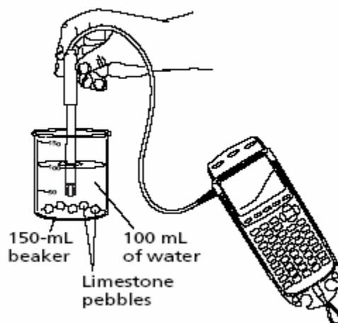
3. Turn on the graphing calculator and start the DataMate program. Press **CLEAR** to reset the program. The pH probe should be recognized automatically. If not, turn to page *vi* for instructions on how to set up the probe manually.
